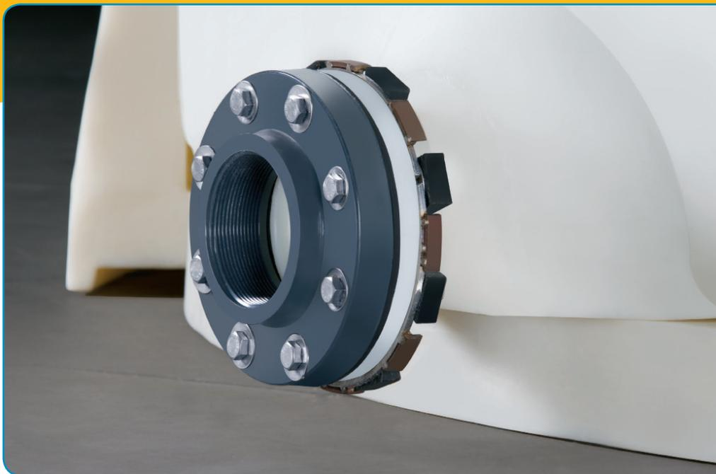
Traditional tank maintenance can be a challenge with many chemicals – so Poly has developed a unique system that helps minimize the hazards associated with traditional vertical tank maintenance. With Poly's Integrally Molded Flanged Outlet, or IMFO® system, the flange is molded while the tank is processing, making it a stress-free part of the tank. The flange is created from the same material as the tank – it's not an insert introduced during or at post-production.
