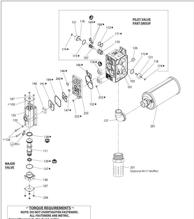
Torque (105) screw to 35 - 40 in. lbs (4.0 - 4.5 Nm). Torque (134) screw to 35 - 40 in. lbs (4.0 - 4.5 Nm).
